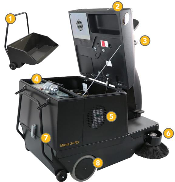
1. The removable 13.2 gallon hopper is equipped with 5 inch wheels to assist the operator when dumping.
