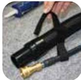
Assemble your vacuum & solution hose. Small loop goes over small hose velcro over large vacuum hose.
