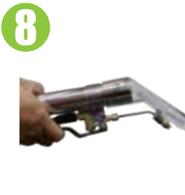
Squeeze hand trigger. Pull trigger until liquid sprays from spray jet. Pump and heater (if equipped) is now primed. With water / cleaning solution.
