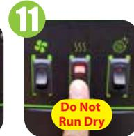
If equipped with a heater. Turn it on for 5-minutes to pre-heat
