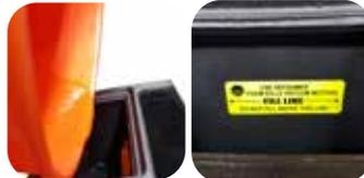
Pour solution into lower solution tank. Access this tank by removing the recovery tank.
