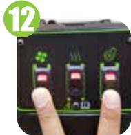
Turn the vacuum and pump motor on. All 3 switches are now on.
