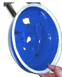
7. Place the Inner Shell back onto the Outer Shell with the rectangular retaining nuts going through the openings in the Inner Shell. The flanges on the Inner Shell set on the edge of the Hard Boot or Brush Ring to hold it in place.
