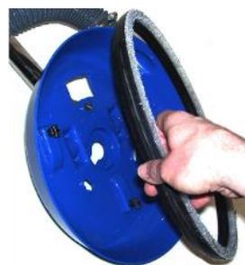
6. Place either the Brush Ring or the Hard Boot on to the bottom lip of the Outer Shell.
