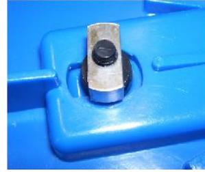
9. Turn the head assembly back over and snap the three retaining levers back down to secure the Outer and Inner Shells. Check the retaining nuts to be sure all three are in contact with the plastic Inner Shell. Open the retaining levers and tighten retaining nuts as needed to assure that the Inner Shell is properly secured when the levers are pushed down.
