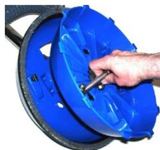
5. Lift up and remove the Hard Boot or Brush Ring from the bottom lip of the outer shell.
