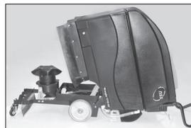
To simplify pad changing, a foot latch at the front of the machine allows the body to tilt up and back. This also provides easy access to the batteries and all internal components.
