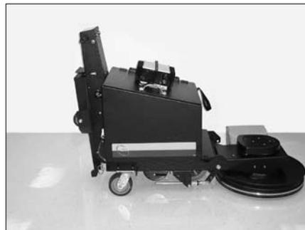
The Sulky flips up 90° from the operating position, allowing the operator to burnish in tight areas.
