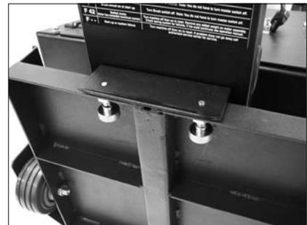
A sturdy, dependable latch holds the Sulky in the "up" position during walk-behind operation.
