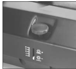
The main brush can be adjusted by turning the knob at the rear of the sweeper. the sidebroom has a separate adjustment.
