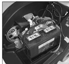
The flip-top battery cover permits easy access to the battery, on-board battery charger, and other internal components.
