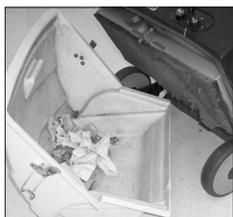
The removable hopper at the rear of the machine makes emptying the Sidewinder 27 MB easy.
