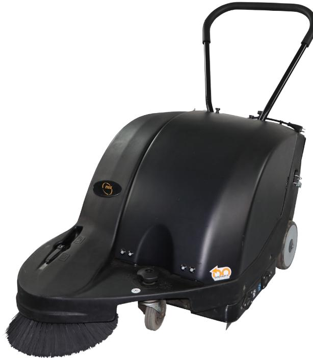
The easy-to-use Sidewinder 27 MB battery-powered sweeper, with its dual counter-rotating brush system, picks up everything from fine dust to large debris in a single pass. Its 27.5-inch (70 cm) sweeping path cleans 15,500 square feet per hour on both carpeted and hard floors, indoors or out.
