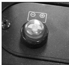
The battery charge indicator light displays battery charge strength during operation.
