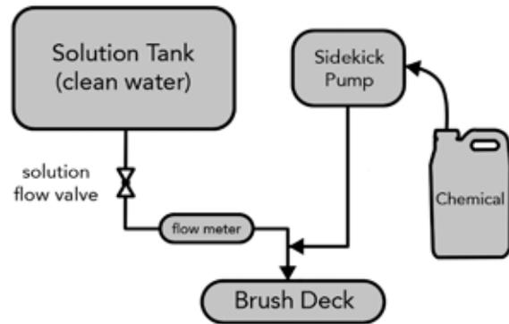
A flow meter in the solution line continuously measures the amount of water used. The Sidekick pump uses this information to send exactly the right amount of detergent to the scrub deck. If the operator changes the water flow, the Sidekick Chemical Metering System automatically adjusts the amount of chemical used.
