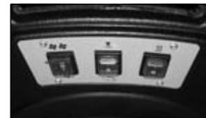
All Predator models are equipped with large, international-symbol rocker switches for easy machine operation.
