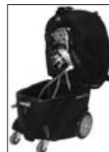
For repairs and maintenance the tip-back feature of the CXH 500 allows easy access to the dual 2-stage vacuum motors, positive-displacement pump, heat exchanger, and other internal components of the machine.
