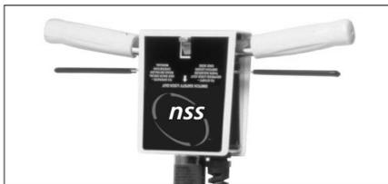
The Mustang 300 DS features a mechanical lock-out which must be released before the switch lever can be activated. This feature helps prevent unauthorized operation.
