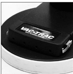
The Mustang 1500 is available with the NSS' Vac-Trac Dust Control System to collect the powder that often results from burnishing old floor finish, and deposits it into a filter at the front of the machine. The filter (#5990291) can be easily removed to clean or replace.
