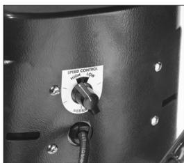
The variable-speed control switch allows the operator to match the pad speed with the job at hand.
