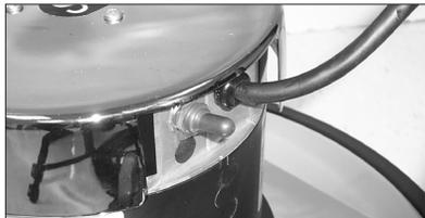
The rocker switch on the rear of the motor permits easy transition from high speed (320 RPM) to low speed (180 RPM).
