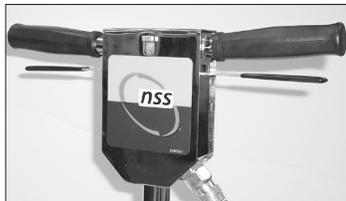
The Galaxy DS features a mechanical lock-out which must be released before the switch lever can be activated. This feature helps prevent unauthorized operation.
