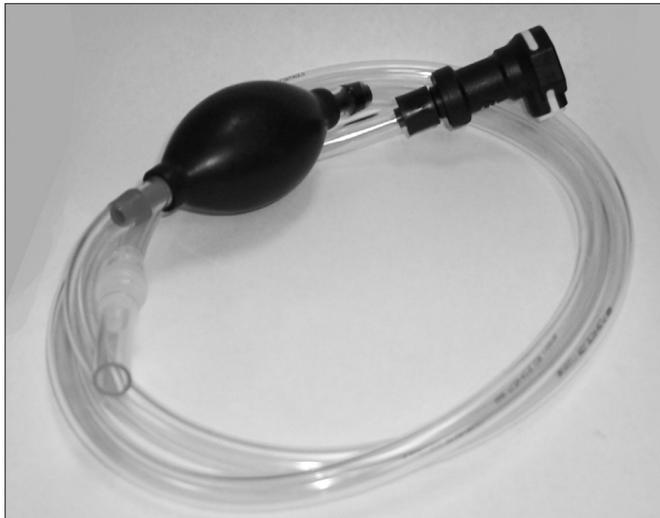
Once the Auto-Fill is completely installed on an NSS machine's battery pack, this hose (connected at one end to a distilled water supply and the other end to the Auto-Fill connector) makes it safe, easy and quick to fill the batteries to their correct fluid level every time.
