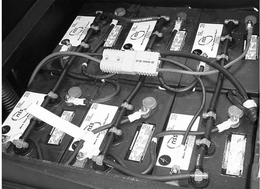
Used conscientiously in an overall battery maintenance program, the Auto-Fill Battery Watering System from NSS® Enterprises, Inc. will extend battery life and reduce machine downtime.
