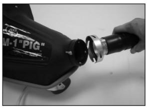
Attach the hose coupling to the machine by slipping it over the locator pins on the intake. Twist the coupling to lock it in place — tighten the wing nuts to secure it. ALWAYS remove the hose and coupling from the machine after each use.
