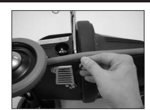
Slide the bottom of the bag rod into the groove in the bottom of the machine, and secure the set screw using the allen wrench provided.
