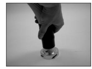
ALWAYS push the hose cuff onto the swivel coupling as far as possible to prevent the hose from pulling off of the swivel when in use. To ease installation you may have to run the hose cuff under HOT tap water for 2 to 3 minutes to soften the hose cuff.
