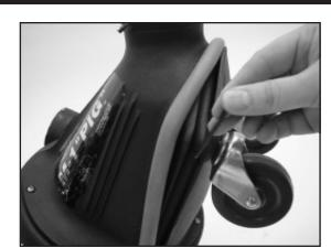
Set screws at the bottom of the machine, under the vinyl bumper, allow the securing or removal of the front casters when replacement is necessary. Lubricate casters as required.
