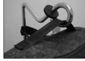
Hang bag strap on the bag rod loop and secure the loop opening with the rubber washer. Attach the bag coupling in the same manner as the hose coupling.
