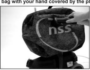
Reinstall the filter bag onto the machine and vacuum the dust from the outside of the filter bag.
