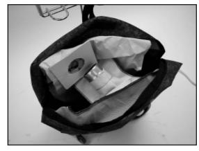
Method #3 A disposable paper bag (#1098861) may also be used inside the filter bag. To empty, pull the disposable bag from the topfilling tube inside the filter bag. Attach another disposable filter bag by pushing the bag opening over the top-filling tube.
