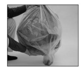
When the filter bag is empty, remove it from the plastic liner. Dispose of the plastic liner. Periodically vacuum the inside of the filter bag for maximum suction and filter bag life.
