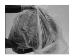
Method #1 Remove the filter bag from the machine and place it into a plastic liner with the coupling at the top. Close the top of the liner around the coupling. CAREFULLY pull the dirt and debris from the filter bag with your hand covered by the plastic liner.
