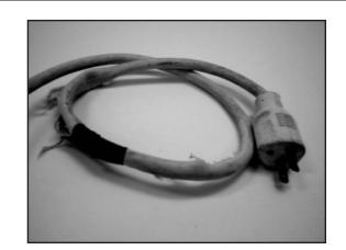
DANGER! Inspect cord daily for wear. When using machine with 2-wire outlets, use a 3-wire/2-wire adaptor plug. Refer to the machine manual for proper grounding instructions. NEVER operate a machine with a cut, abraded or taped cord, or with a broken grounding pin. These conditions can result in electrical burn, shock or electrocution to the operator or bystanders. Always replace damaged cords to maintain safe operating conditions.
