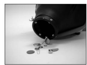
Dump out the scrap trap frequently to prevent fan damage caused by overfilling the scrap trap with debris.
