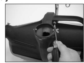
Remove screw from the top bag rod post. Insert the top bag rod post into the hole in the handle. Replace and retighten the screw into the top bag rod post.
